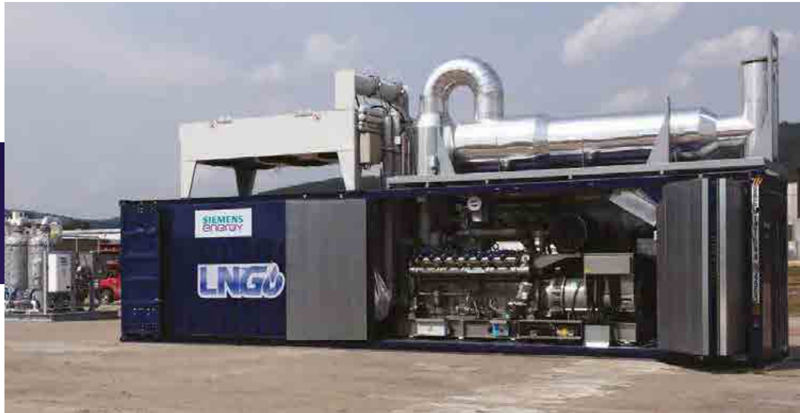
LNGo micro-scale natural gas liquefaction system.
